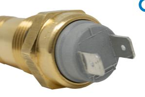
Use these Temperature Switches to control oil temperature by cycling the cooling fan to maintain the desired entering, or leaving temperature. The temperature switches are designed to be installed in the drain ports of the DC fan Series Coolers. It is a normally open switch that closes on temperature rise. We recommend relaying and fusing the temperature switch and fan.
