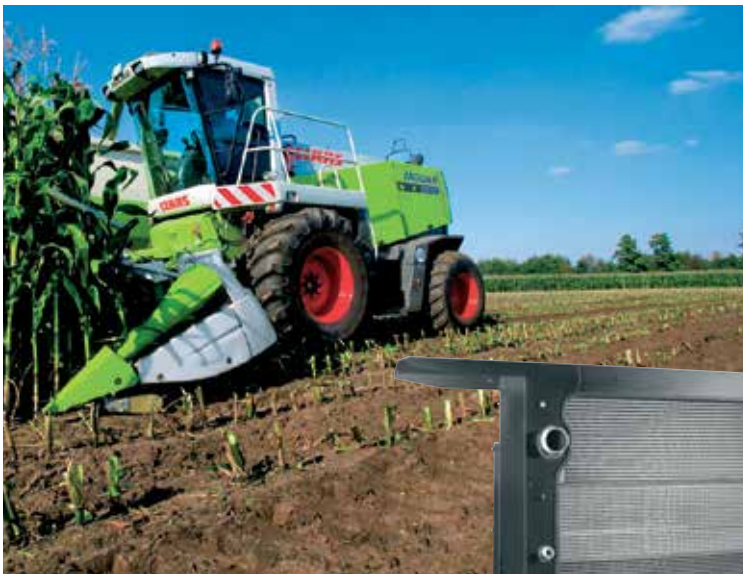
Combination Coolant/ Charge-Air and Oil Cooler for the „Jaguar 900“ Forage Harvesters, Claas
