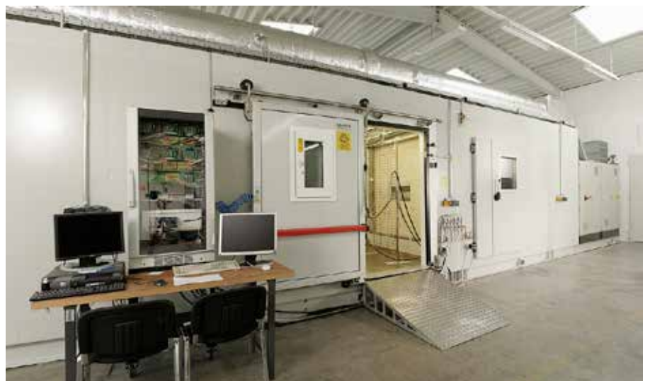
Wind tunnel for performance measurement of large cooling systems
