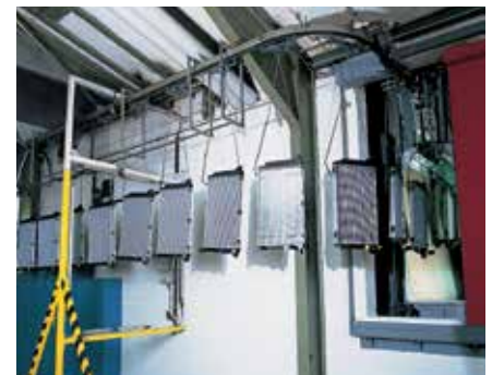
Electrostatic paint line
