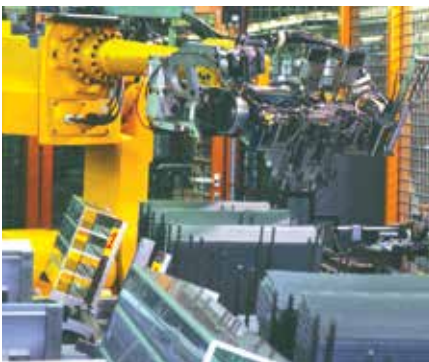
Robot for the assembly of cooling cores
