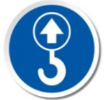
Figure 2: Mandatory action: lifting point location. Label present on all AKGTS catalog standard cooler assemblies with provided lifting eyes.
