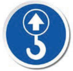
Figure 2: Mandatory action: lifting point location. Label present on all AKGTS catalog standard cooler assemblies with provided lifting eyes.
